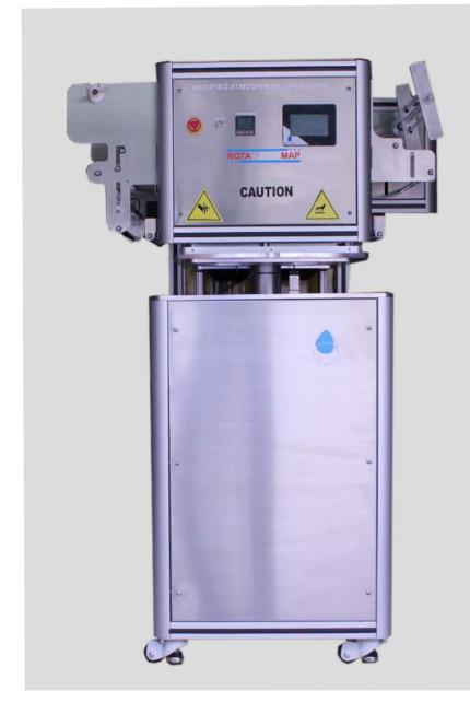
The two station rotary tray sealers are specially designed for Modified Atmosphere Packaging. Simple interface, variable controls and easy tool change makes operation more easier.
